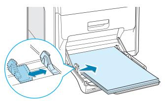
If you want to print on previously printed paper from the Multi-purpose Tray, the printed side should be facing up with the uncurled edge towards the printer. If you experience problems with the paper feeding, turn the paper around.
